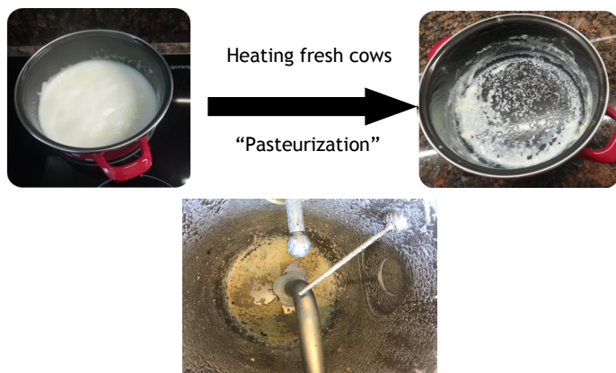
Figure 1: Top - Coagulation of milk proteins and formation of the deposit on the bottom of the pot. Bottom - Fouling in the pilot plant, deposit formation in flash cooler.
